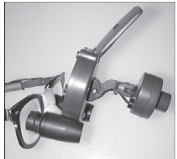
Figure 3. Wireless X10 VHS Cam mounted to surgical loupes.
